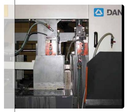
For precision, the Danobat's movable arm automatically adjusts to the width of the material.
